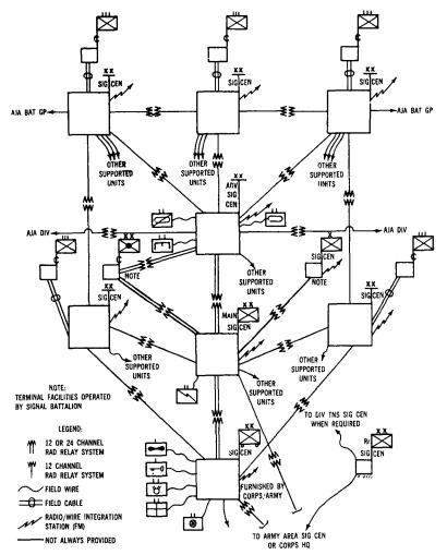
Figure 5. Type infantry division area communications system. (Schematic only. Troop dispositions, operational requirements, enemy capabilities, and other factors dictate the configuration.)
